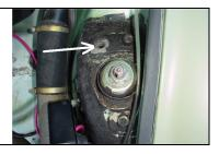
2 – Using the longer 10 mm socket cap screw and one Belleville washer provided, loosely assemble the driver side tower as shown. Orient red ends so the red mark is up.
