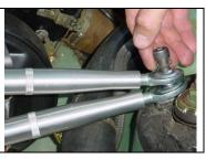
3 – Using the shorter 10 mm socket cap screw and one Belleville washer provided, loosely assemble the passenger side tower as shown. Orient the rod end with the red mark up. The knurled end of the braces must be on the driver's side.
