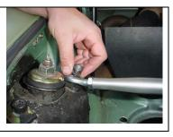
4 – Inspect trunk floor to determine if an existing hole is in place to secure the diagonal brace. Cars built before 1978 should have the hole, it may be filled with a plastic plug that must be removed. The hole should be positioned as shown.
