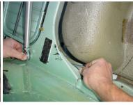
6 – Tighten shock tower socket cap screws to 34 ft/lbs using an 8mm hex key. Tighten the trunk floor socket cap screw to 60 ft/lbs.
