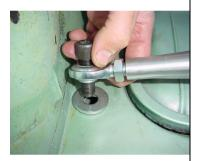
The following technique can be used to position the nylock nut and washer. Using low-tack tape, loosely affix the nylock nut and washer to a long-handled open-end wrench as shown.
